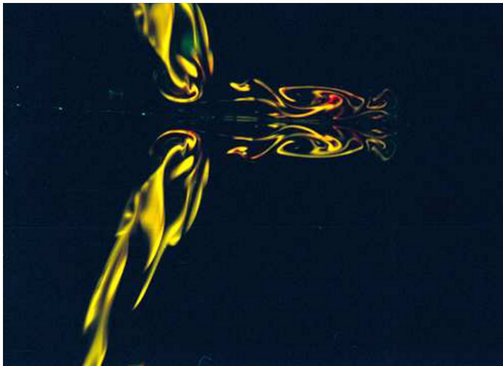
Fig. 2. Laser induced fluorescence of buoyant rhodamine plume impinging on free water surface. Sarah Stapleton, by permission.
