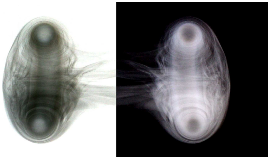
Fig. 7. Vortex ring in air, visualized with stage smoke. Emrys Hall, Thomas King, Bethany Rotherham, Brynne Sutton, by permission.
